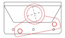
Mark the middle point of the bushing on each bracket. Drill an 8mm hole at the marked position into each bracket and smooth the edges.
