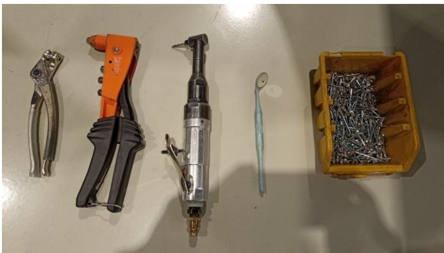
Fig. 5 Tools needed to install missing rivets. Refer to 3.2
