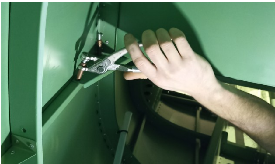
Fig. 11 Remove the clecos by pliers. Then install remaining rivets.
