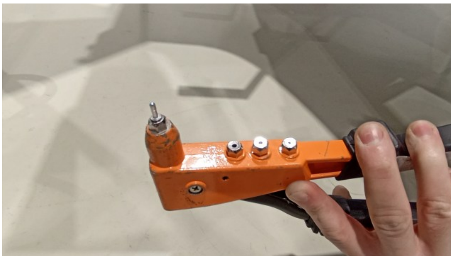
Fig. 8 Insert the rivet into hand riveter
