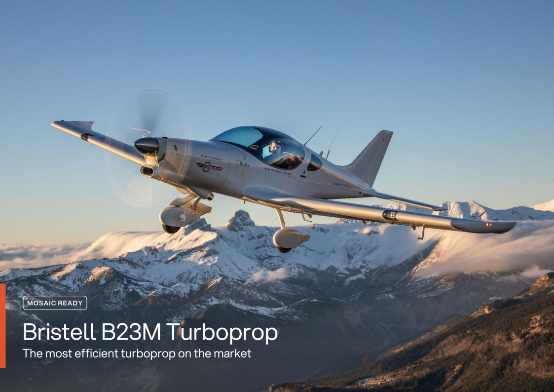
The Bristell Turboprop, powered by the Turbotech turbine from France, is the perfect solution for powering light airplanes. Turbotech specializes in lightweight turbines with highly efficient fuel consumption. Thanks to its special heat exchanger, the turbine's fuel consumption is comparable to that of the most powerful four-cylinder combustion engines.
