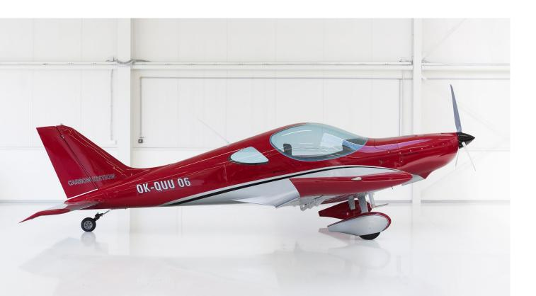
Bristell Taildrager option with the Busch wheel variant, featuring the robust Busch landing gear from the Beringer company. With a combination of the Rotax 916iS and a constant speed propeller, the takeoff distance is less than 300 feet. Let's go enjoy Busch flying in the most comfortable LSA on the market.
